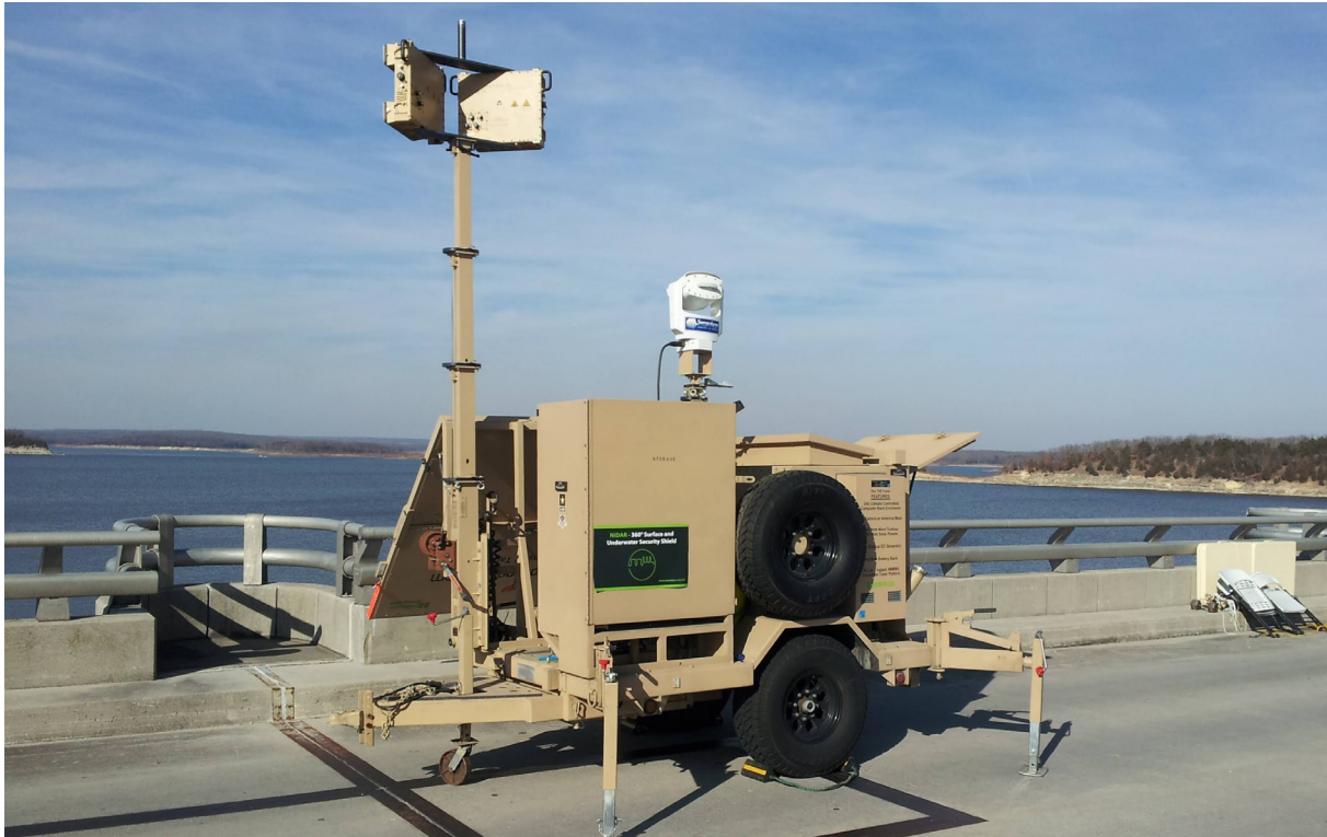
Figure 4: Blighter radar deployed on solar-powered trailer system
